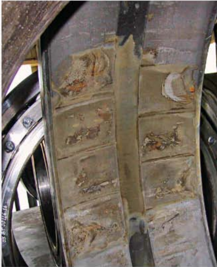
The outer race of a spherical roller bearing in need of bearing remanufacture.
