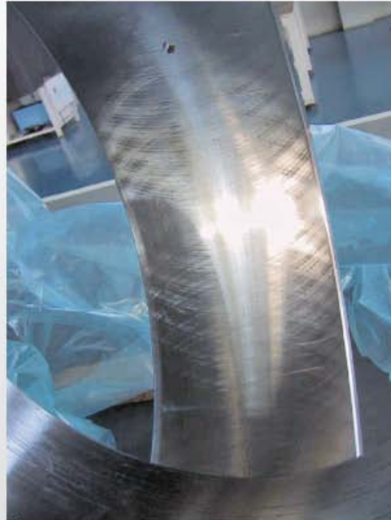
The outer race of a large spherical roller bearing after remanufacture, which includes the process of removing aggressive surface damage by using a grinding or hard-turning process.
